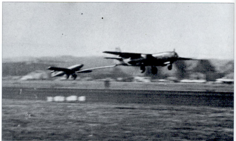
Test flight by a development Arado Ar 234 towing a Deichselschlepp (air trailer) auxiliary fuel tank. Ken Ellis collection
